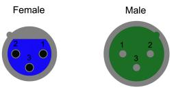
By convention, the two signals are referred to as the positive phase (sometimes referred to as 'hot') and the negative phase ('cold').
