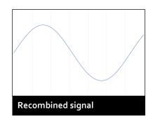
Now when the two wave forms are recombined (by subtracting one from the other), the noise cancels itself out, leaving the original, noise-free signal.
