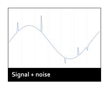
Unfortunately, once the signal has become corrupted with noise, there is no method of removing this noise without further damaging the original signal.
